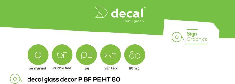
Vinyl for decorating glass or glazed surfaces indoor and outdoor, with 80 mic polymeric PVC film, bubble free high tack, high cohesion permanent adhesive and 145 gr Clay coated PE embossed paper liner.
